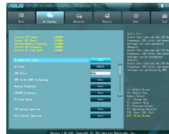
9. Enable A.M.P. Memory Profiles to set Memory Frequencies. For those without AMD Radeon™ Memory, enable XMP in the BIOS (See image at right) to ensure maximum memory settings.
